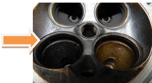
Figure 3. Traces of abnormal contact of the intake valve with the inner edge of the seat (left), which indicates valve head deformation.
