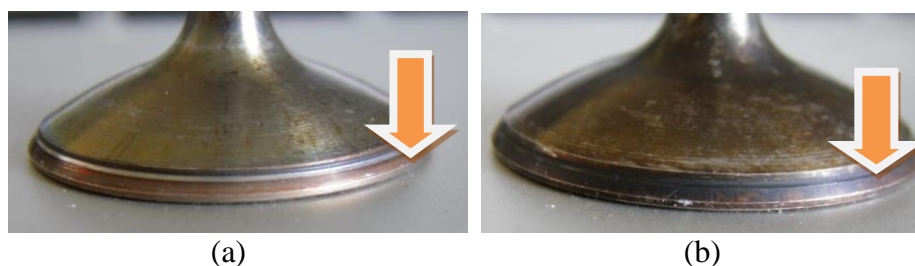
Figure 2. Valve head deformation causes its shift to the inner edge and a substantial reduction in the width of the contact line with the seat (a), which then leads to severe wear of the valve face and full loss of contact with the seat (b).
