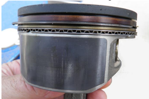
Fig. 10. A normally working piston always has the top land area evenly covered with soot around the entire circumference.
