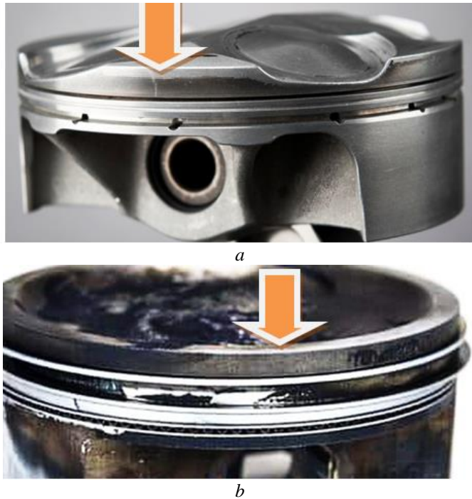
Fig. 13. Small two-sided marks of scuffing over the pin holes on the top land of sports engine pistons – from a slight touch (a) to a wide contact area (b).
