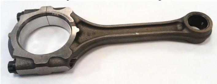
Fig. 1. A typical traditional conrod with the I-beam stem.
