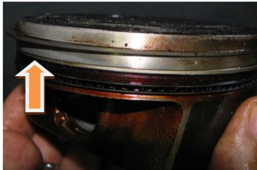
Fig. 12. A typical and clearly marked one-sided wear of the piston top land over the pin hole is caused by the work of the piston with an inclination.
