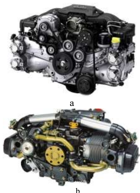
Fig. 2. Engines: a – Subaru car engine has examples of aviation applications; b – Limbach aircraft engine, created by the deep modernization of the old automotive boxer engine VW
