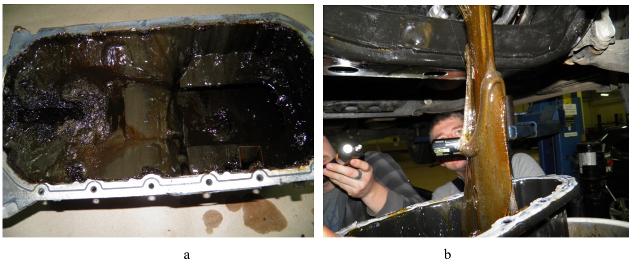
Figure 3 – Typical examples of changes in the properties of motor oil when exposed to low-quality fuel: sediment formation (a) and its transformation into a rubbery mass (b)
