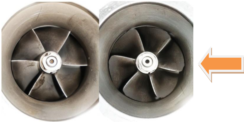
Fig.2.2. Selective gas-abrasive wear of the inlet edges of the compressor blades of one of two turbochargers over 42000 km of vehicle mileage [9]
