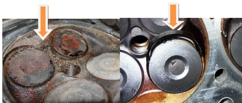
Fig.4.2. A combustion chamber with traces of melting of the wall between the exhaust valve seats, damaged during the nominal operating mode of the internal combustion engine in motion (a), and a case of overheating with seats falling out due to loss of coolant at low speeds and loads when the internal combustion engine is operating at a standstill (b)
