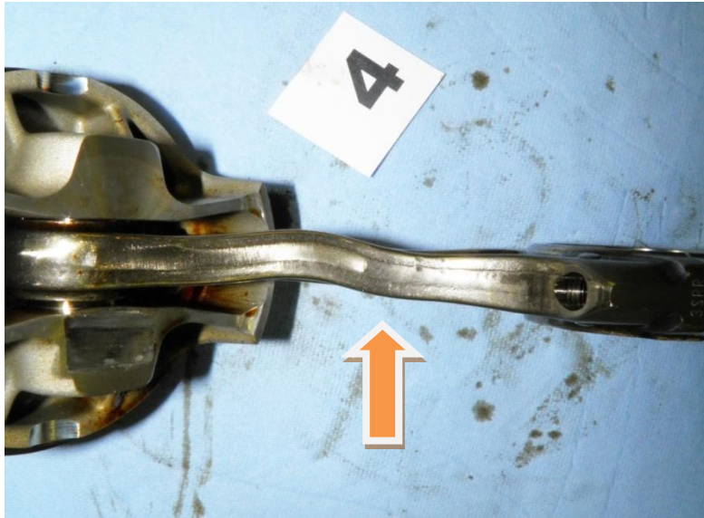
Fig.3.1. The typical shape of the connecting rod stem in the hydrolock in the cylinder after loss of stability
