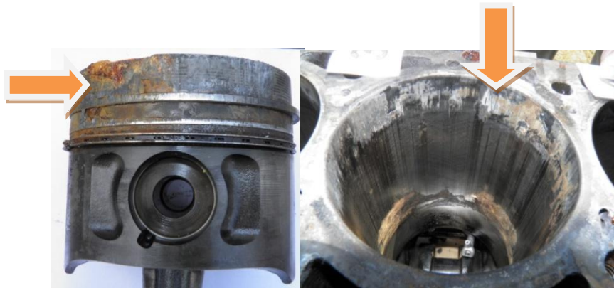
Fig.4.5. Seizures in the upper part of the piston (a) and on the cylinder (b) from diesel overheating due to loss of coolant. The traces of gas breakthrough on the upper cylinder block surface are clearly visible [35]
