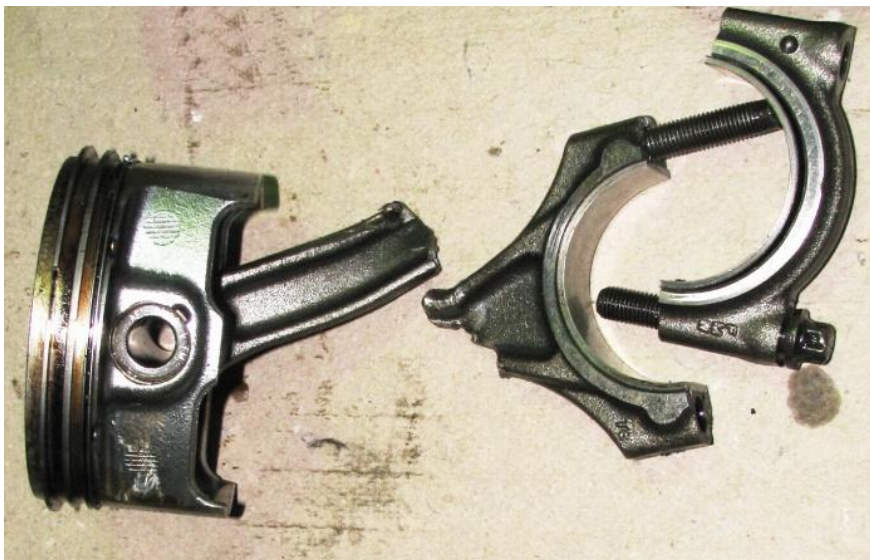
Fig. 3.2. Fatigue failure of the connecting rod after hydrolock does not allow any data to be obtained using direct measurements of the rod
