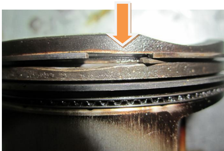
Fig.2.4. Extremely strong selective (local) abrasive wear of piston No. 1 over 80000 km, while there is almost no wear on other cylinders
