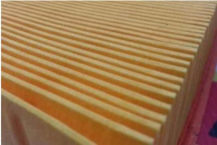
Fig.2.6. Traditional paper air filters are based on particle retention using a sieve effect
