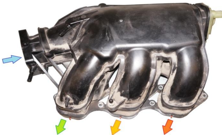
Fig.2.3. Intake manifold with variable channel length for a V-6 gasoline engine
