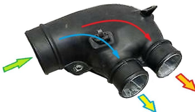
Fig.2.1. A pipe with flow branching from the air filter to the turbochargers of the right and left rows of cylinders of V-diesel engine
