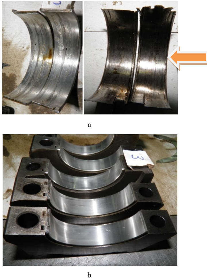
Fig.5.1. A typical example of damage to the connecting rod bearings (a) in the absence of noticeable damage to the main bearings (b) is a common result of operating an engine with insufficient oil levels
