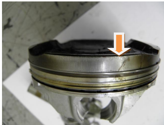
Fig.3.4. Typical traces of piston operation with distortion in the cylinder after hydrolock
