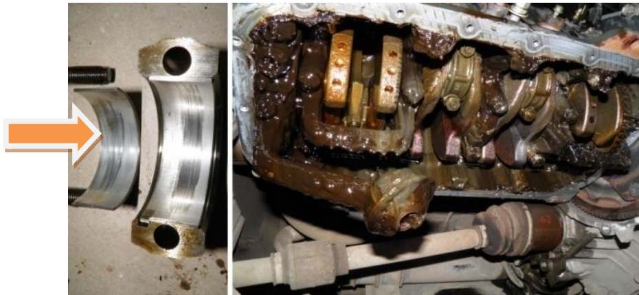
Fig.5.2. The opposite case is damage to the main bearings through melting, jamming of the shaft and rotation of the bearings in the cylinder block (a). Damage to the main bearings was accompanied by relatively minor damage to the conrod bearings (b) and was caused by extremely rapid degradation of the engine oil with clogging of the oil receiver screen
