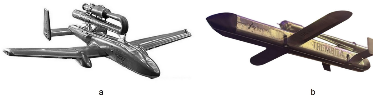
Fig. 1. Some modern unmanned aerial vehicles with a pulse jet engine: (a) Scitor from Wave Engine Corporation, USA (Wave Engine Corp. 2025) and (b) Trembita from PARS, Ukraine (Wikipedia 2025c).
